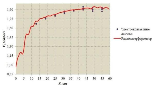
**Figure 4.**  $V-X$  diagram for the movement of the flyer accelerated RDX-based HE explosion products
