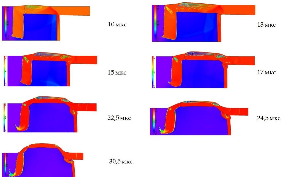
**Figure 7.** Spallation of the body and closure of spalls
