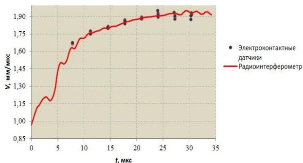
**Figure 3.**  $V-t$  diagram for the movement of the flyer accelerated RDX-based HE explosion products
