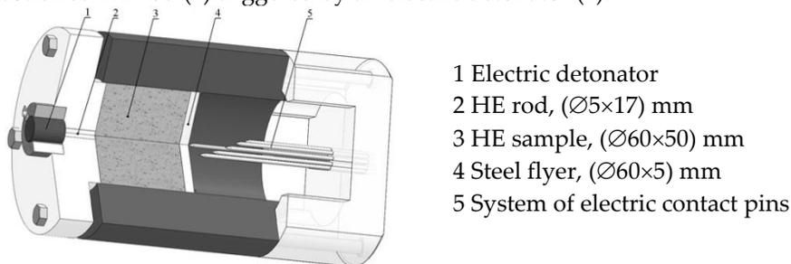
**Figure 1.** Schematic experimental assembly with electric contact pins according to the M-60 technique
