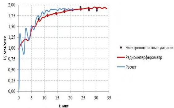
**Figure 8.** Flyer velocity versus time
