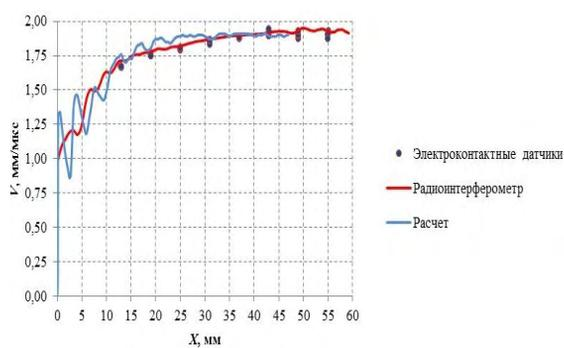
**Figure 9.** Flyer velocity versus coordinate
