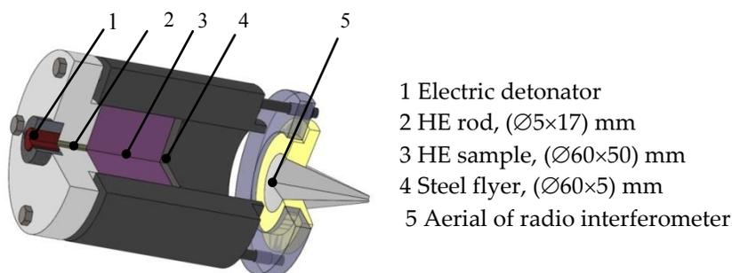
**Figure 2.** Schematic experimental assembly with the radio interferometer according to the M-60 technique
