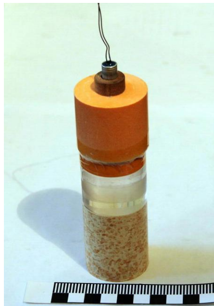
1 – electric detonator with a plug fixation; 2 – plane wave generator; 3 – initial charge; 4 – Plexiglass barrier; 5 – test (inert) charge; 6 – witness plate.
