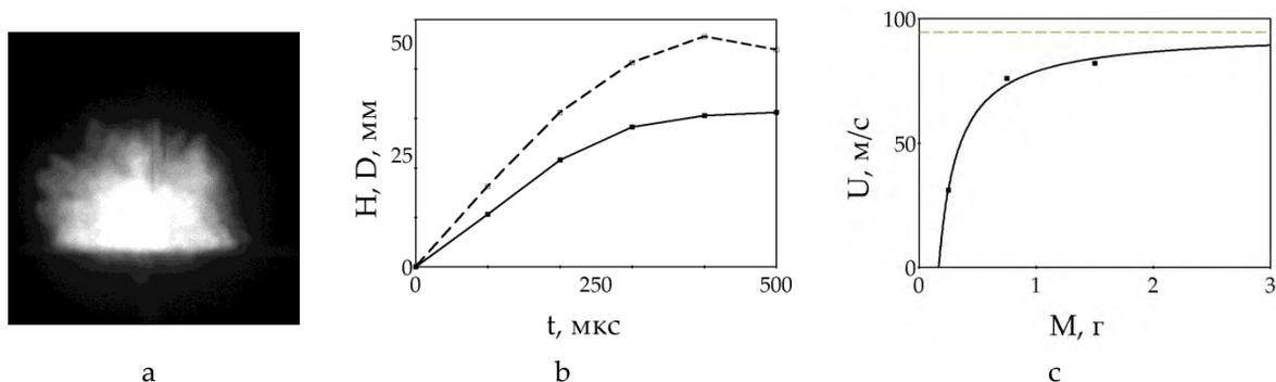
**Figure 3.** a – The photo of light emission area under natural expansion of cold components and reacting clusters (0.3 g) along and across the flat base; b – timing diagram of the diametrically (dotted line) and vertical (solid line) expanding of the light emission area; c – dependence between the vertical velocity of light emission area and the mass of sample
