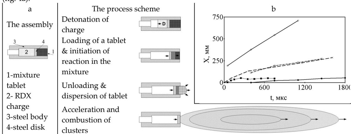
**Figure 4.** a – A scheme of the experimental assembly and the process of impact loading: 1 – extruded mixture tablet, 2 – RDX charge (1.15 g/cm<sup>3</sup>), 3 – intermediate steel disc, b – The time diagrams of different regions of the light emission area: 1 - flow front; 2 - stream center; 3 – plasma front; 4 - the stream radius; 5 – flow rear area
