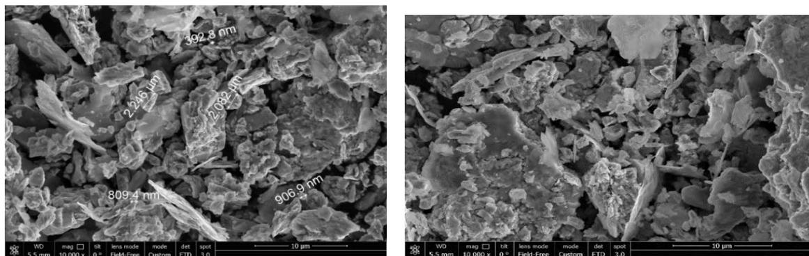
**Figure 1.** Microscopic photos of Al and CuO powders mixture
