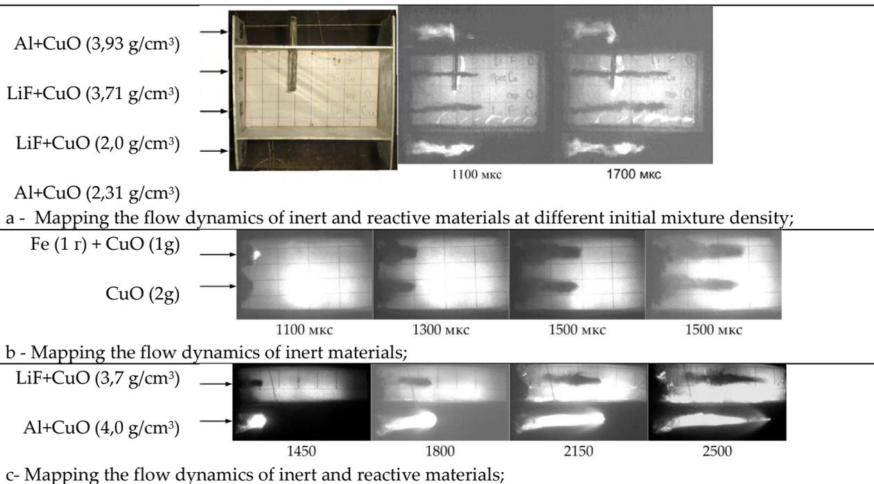
**Figure 6.** Photos of flows of various powder materials
