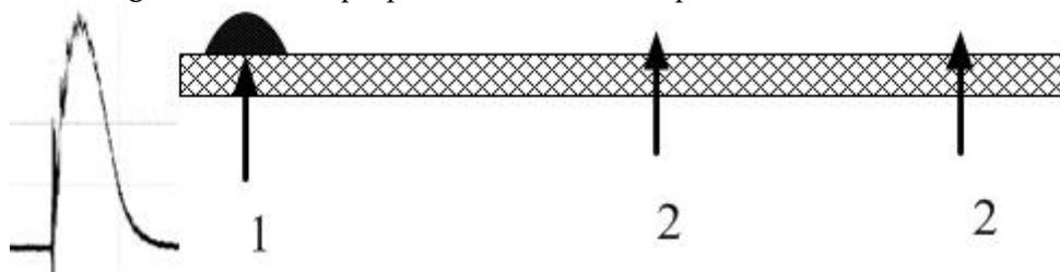
**Figure 2.** The waveform of spark current and the scheme of experiment with electric-spark initiation. 1 – Current electrodes; 2 – Electric sensors
