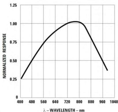
Figure 5. Spectral sensitivity of the time interval recorder (TIR)
