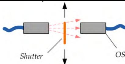
**Figure 11.** Measurement of the mechanical-system state variation rate
