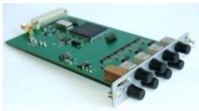
Рисунок 4. Appearance of the time interval recorder
