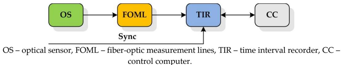
**Figure 1.** Schematic measurement channel of the multi-channel system
