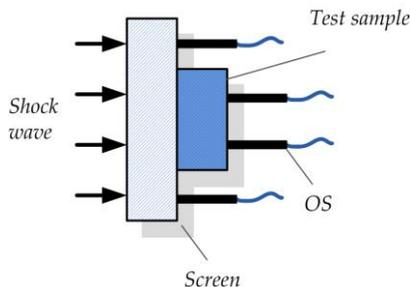
**Figure 8.** Measurement of shock-wave velocity
