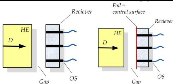
**Figure 9.** Measurement of times of the shock-wave arrival into the gap and at the test surface
