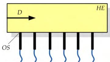
**Figure 7.** Measurement of detonation velocity
