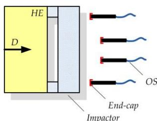
**Figure 10.** Measurement of impactor velocity
