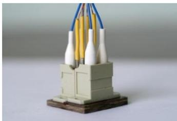
**Figure 2.** A sample assembly to measure the air shock-wave velocity
