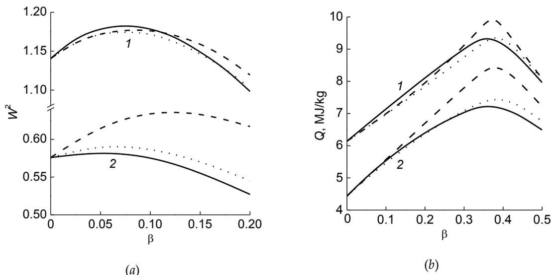
**Figure 4.** (a) – AA, (b) – HoE for the compositions based on HEs: 1 – CL-20, 2 – TNT versus the Al concentration. The designations are the same as in Figure 3
