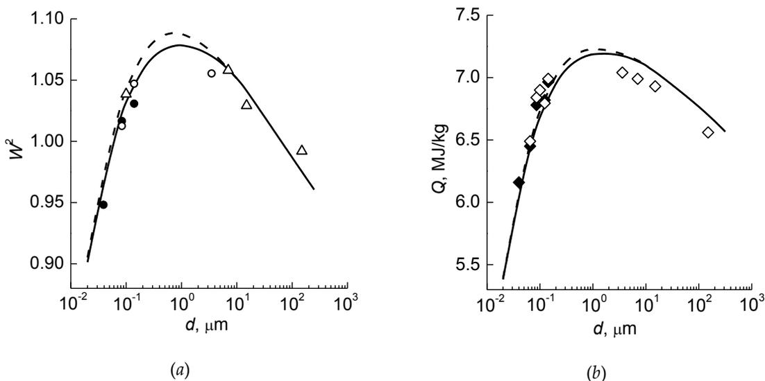
**Figure 1.** (a) – AA, (b) – HoE of the HMX-based compositions versus the Al particle size after the addition of 15% Al; solid lines – mechanical mixtures, dashed lines – nanocomposites; circles – M-20, triangles – M-40, rhombuses – HoE
