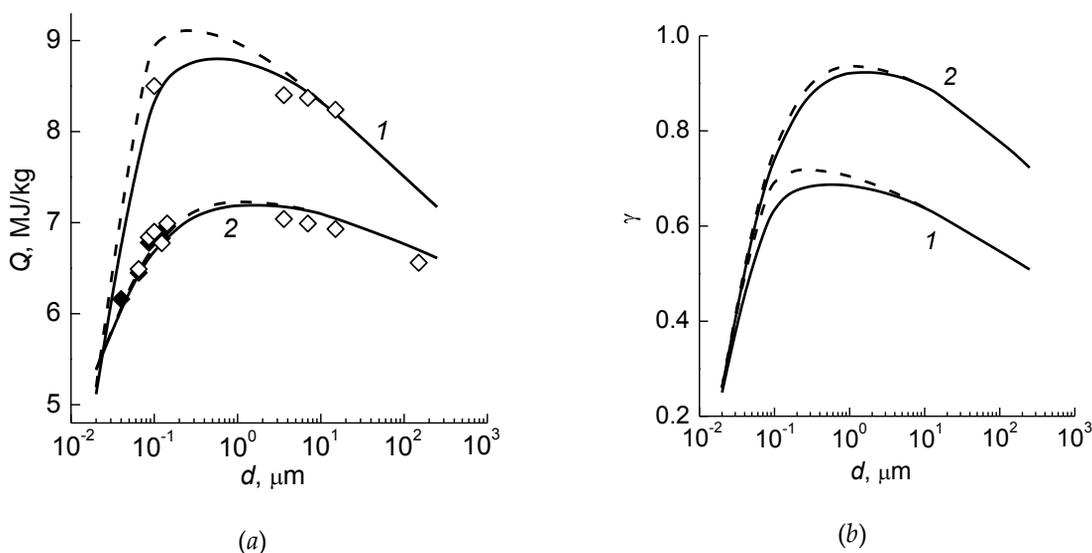
**Figure 2.** (a) – HoE, (b) – the degree of the Al additive oxidation for the HMX-based compositions versus the Al particle size after the addition of 15% (1) and 40% (2) Al. The designations are the same as in Figure 1
