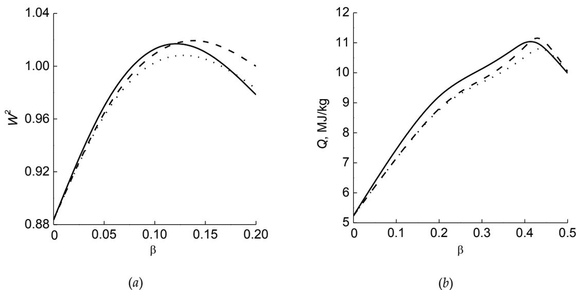
**Figure 3.** (a) – AA, (b) – HoE for the BTNEN-based compositions versus the Al concentration; solid lines – mechanical mixtures with Al(7), dotted lines – mechanical mixtures with Al(0.1), dashed lines – nanocomposites with Al(0.1)
