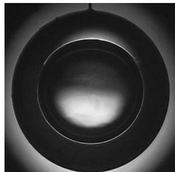
Fig. 2. Cryogenic layer of deuterium in the spherical shell
